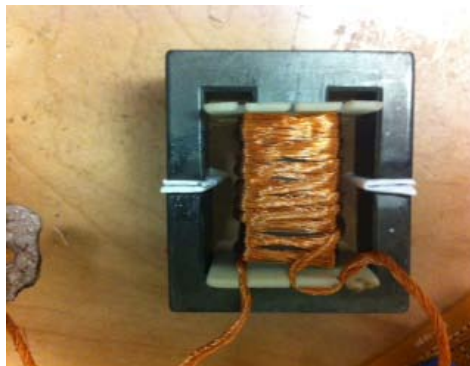
Fig. 6.19 5 \mu H auxiliary inductor
