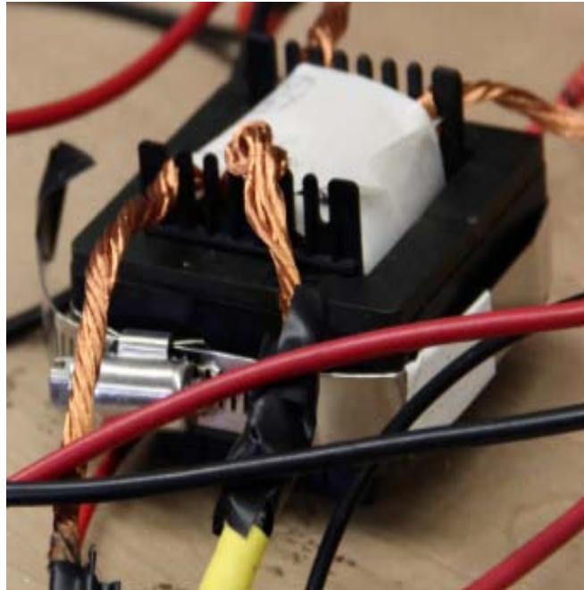
Fig. 6.14 1 kW high frequency transformer
