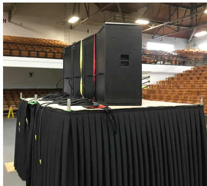
Point source speaker cabinets on scaffolding. Each box weighs 250 pounds and can use over 6000 watts of power.
