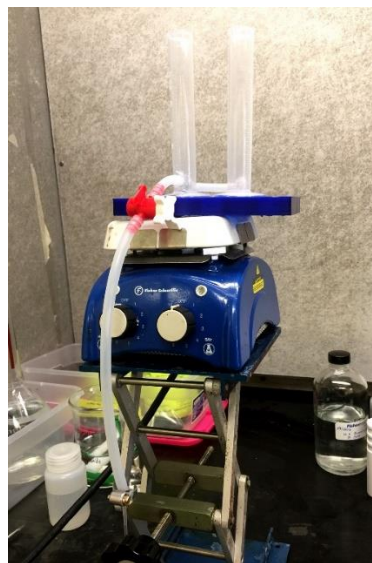
Figure 2. Gradient Former Constructed for Experiments. Image of the constructed gradient former as it appears during an operation to cast a gradient gel.
