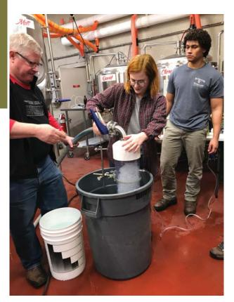
Annelies van der Bleek setting up a test column at Red Silo Brewery. Red Silo helped students create nitrogen-saturated spring water in their brewing room.
